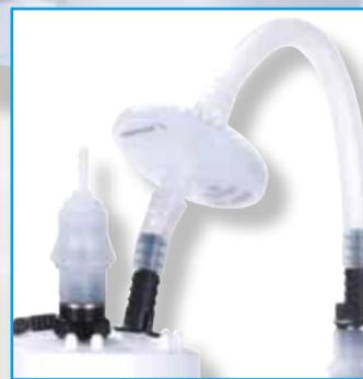
Filter 0.2 micron - high protection against contamination, autoclavable
