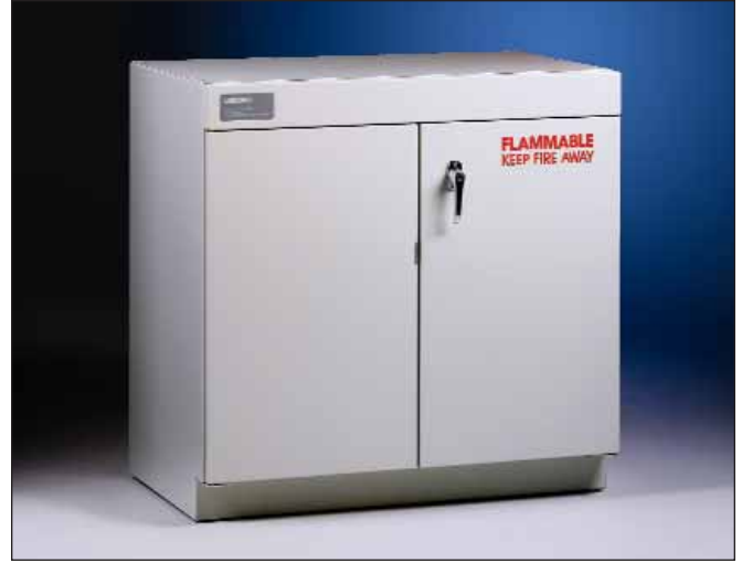
Protector Solvent Storage Cabinets have dual wall epoxy-coated steel construction with 1.5" air gap. They include an epoxy-coated steel interior shelf and two rear vent connections with flame arrestors and closure plugs.
