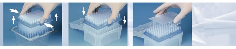
Press the long sides of the transfer aid together, and continue pressing them together while withdrawing the tip-tray. Ensure that the holding straps for the transfer aid are correctly positioned. Insert the filled tip-tray perpendicularly from above into the previously sterilized TipBox until it locks into place.
